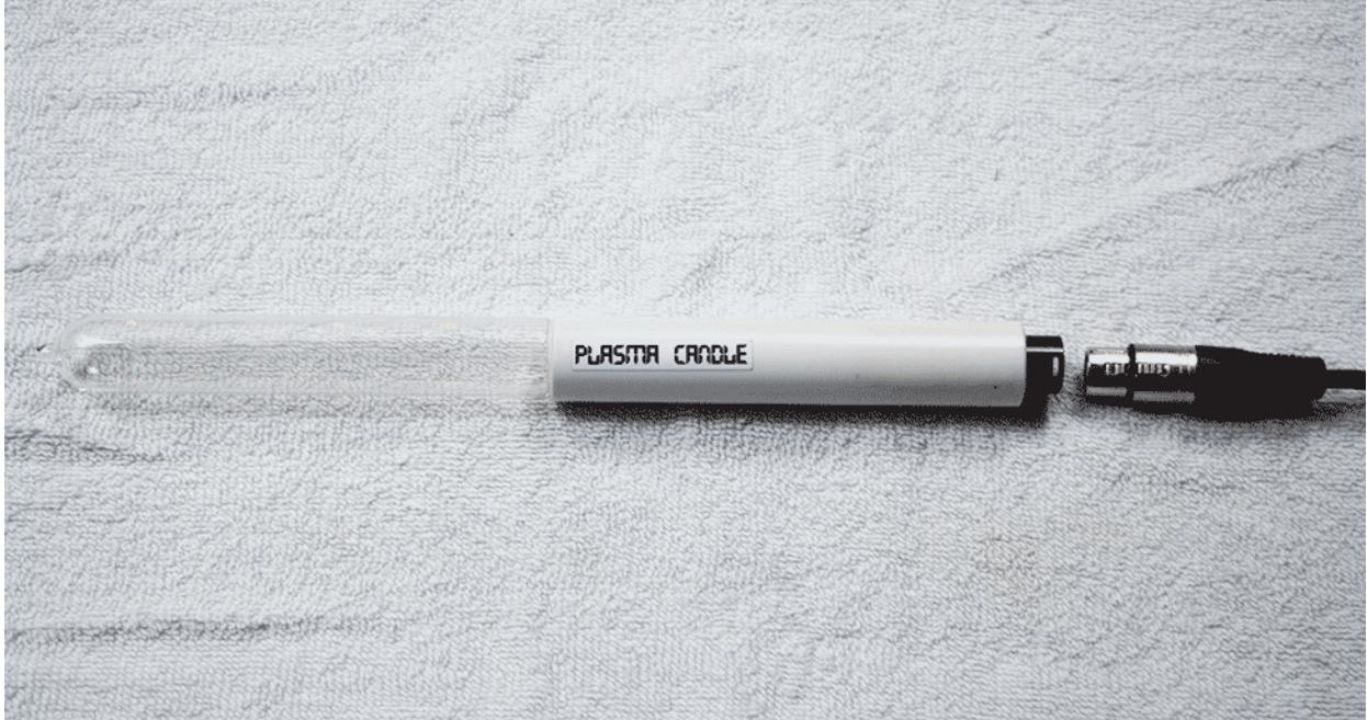
If you have the Plasma Candles, plug the female end of the audio cable into the bottom end of the candle. Push the plug all the way into the socket until you hear a click.
