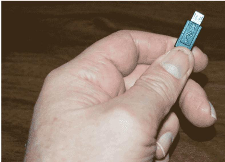
Pick up the small end of the supplied USB cable. Orient the end so that the side with the black dot is facing down.
